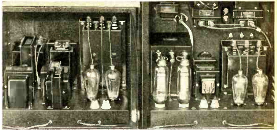
Rear view of the R.F. power supply and the modulator in their cabinets. Note that all the units for the modulator smoothing circuit are attached directly to the upper 8 3/4"x17" panel. The tubes to the right are the 66 rectifiers and those to the left are the RK-31s. Except for the resistors and filter condensers, everything used in the R.F. power-supply may be seen in this rear view. The "heavy-duty" sub panel holds it all.
